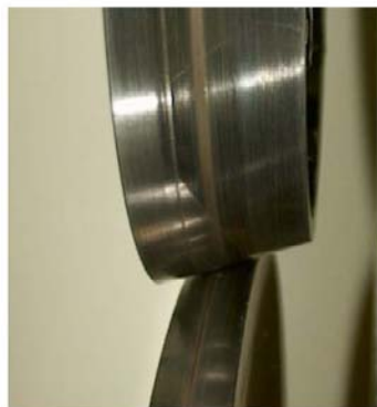
Figure 1: Different contact shape considering a conical (0.3 rad) wheel over a rail (transversal curvature radius 0.06 m) or a roller (0.06 m and 0.025 m).
