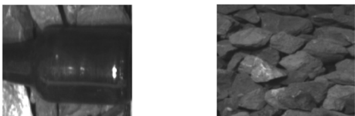
Figure 3: Examples of 160x160 pixels patches: foreign object (left) and ballast (right).
